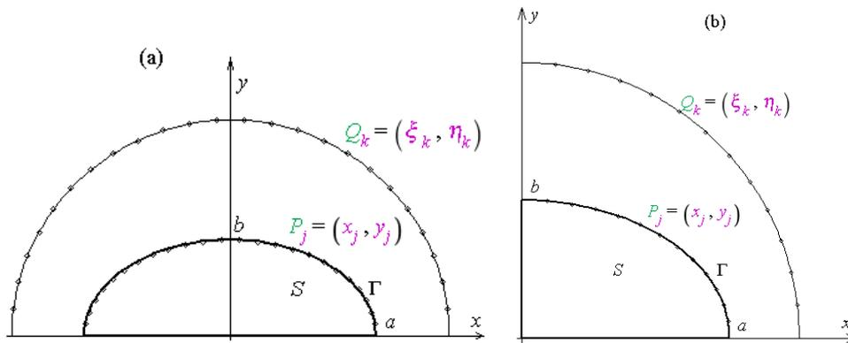
Fig. 1. Geometry configuration of the considered domains with collocation points  $P_j$  on the elliptical arch and source points  $Q_k$  on the circular arch; a) half-ellipse domain, b) quarter-ellipse domain
