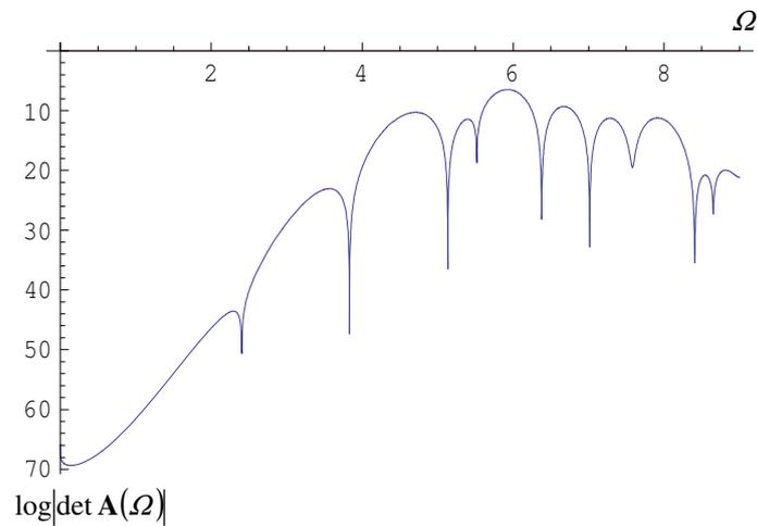
Fig. 2. Logarithmic values of modulus of the determinant  $\det \mathbf{A}(\Omega)$  as a function of  $\Omega$  for the Helmholtz operator in the elliptical domain with semi-diameters ratio  $a/b = 2.0$
