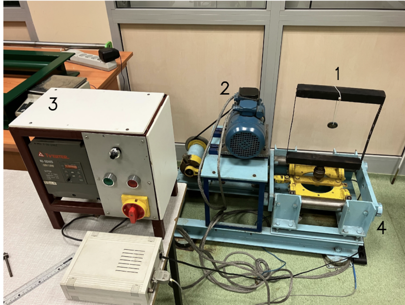
Fig. 2. Physical model of a skyscraper utilizing a dynamic vibration absorber with a variable pendulum moment of inertia. Legend: 1 – model of a skyscraper with a pendulum, 2 – electric motor, 3 – frequency inverter, 4 – shaking table
