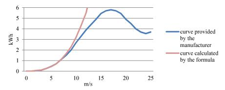
Fig. 5. Wind turbine power, read from the graph given by the manufacturer, compared with the power calculated by the formula [10-12]
