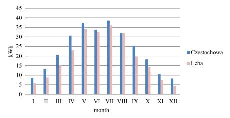
Fig. 4. Electrical energy generated by a single photovoltaic panel within a month in Czestochowa and Leba [own calculations]
