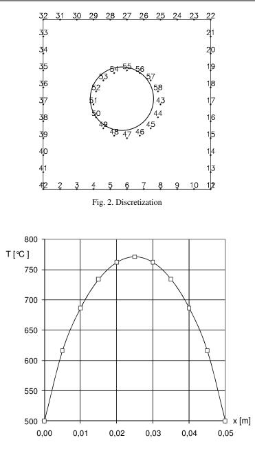
Fig. 3. Temperature distribution along the bottom surface
