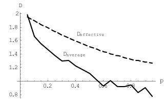
Fig. 3. Solid (dashed) line presents the changes of the average (effective, from analytical calculations) diffusion coefficient D as a function of the conditional probability value p
