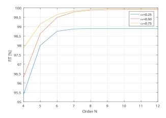
Fig. 2. The fitting of approximation (19) to analytical solution (17) as a function of ORA approximation order N for different orders  $\alpha$ , the bandwidth W = 4
