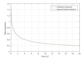
Fig. 1. The comparison of approximated (19) to analytical step response (17) for  $\alpha = 0.5, N = 8, W = 4$
