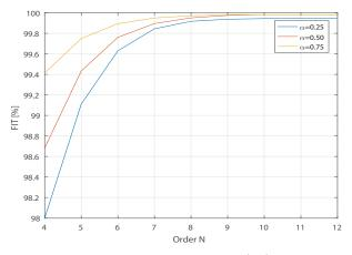
Fig. 6. The fitting of approximated module  $M_{ORA}(j\omega)$  to analytical one (24) as a function of N for different  $\alpha$ , W = 4
