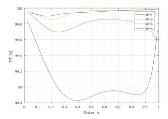
Fig. 5. The fitting of approximated module  $M_{ORA}(j\omega)$  to analytical one (24) as a function of bandwidth W for different orders  $\alpha$
