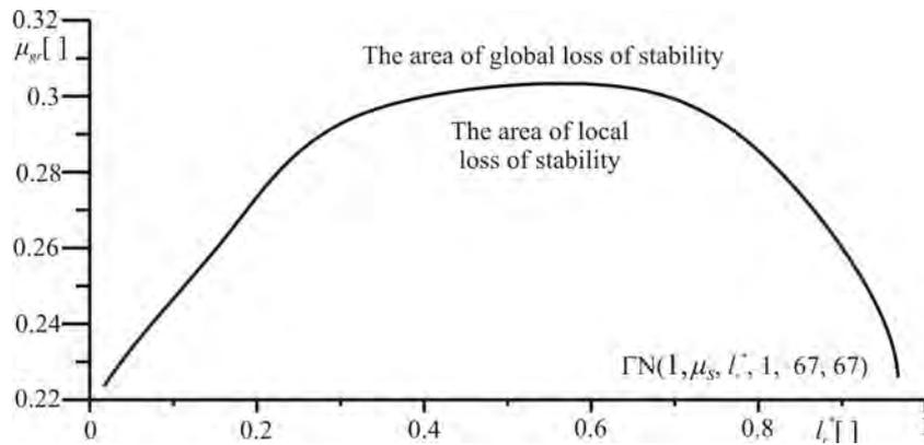
Fig. 8. The influence of the value of loading and receiving heads radius  $R$  on the limit value of coefficient of the flexural stiffness asymmetry  $\mu_{gr}$
