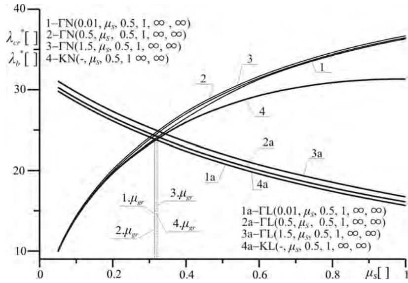
Fig. 4. The critical load parameter  $\lambda_{cr}^*$  ( $\Gamma L$  frame) and the bifurcation load parameter ( $\Gamma N$  frame)  $\lambda_b^*$  as a function of coefficient of the flexural stiffness asymmetry of frame column  $\mu_s$  for different values of coefficient of the flexural stiffness asymmetry of total system  $\mu_C$
