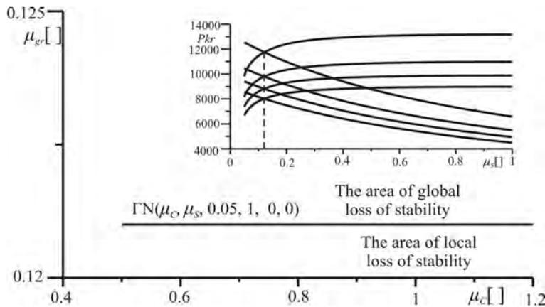
Fig. 7. The influence of coefficient of total flexural stiffness asymmetry  $\mu_C$  on the limit value of coefficient of the flexural stiffness asymmetry  $\mu_{gr}$  of the frame column of  $\Gamma N$  system, where  $c_1^* = 0$  and  $c_2^* = 0$
