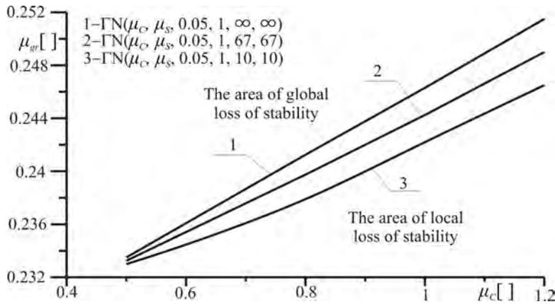
Fig. 6. The influence of coefficient of total flexural stiffness asymmetry  $\mu_C$  on the limit value of coefficient of the flexural stiffness asymmetry  $\mu_{gr}$  of frame column of  $\Gamma N$  system for selected values of the frame column and bolt mounting rigidity coefficients  $c_1^*$  and  $c_2^*$
