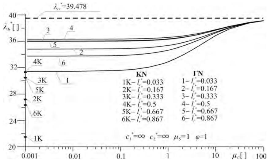
Fig. 9. The values of bifurcation load parameter  $\lambda_b^*$  as a function of coefficient of total flexural stiffness asymmetry  $\mu_c$  for selected values of radius of loading and receiving heads parameter  $l_r^*$
