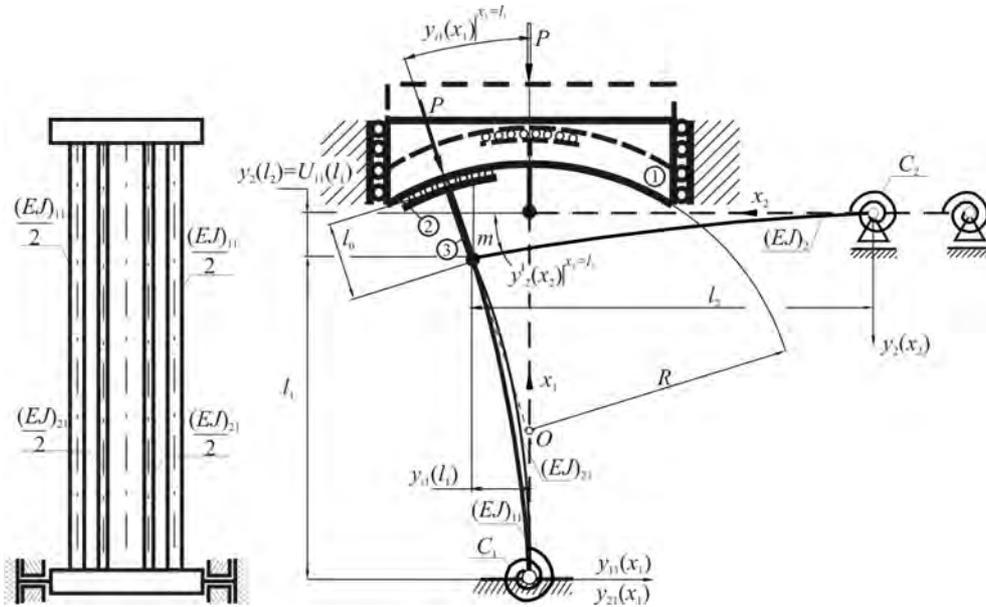
Fig. 1. The flat frame of  $\Gamma$  type with a geometrically nonlinear frame column subjected to the follower force directed towards the positive pole  $\Gamma N(\mu_C, \mu_S, l_r^*, \varphi, c_1^*, c_2^*)$
