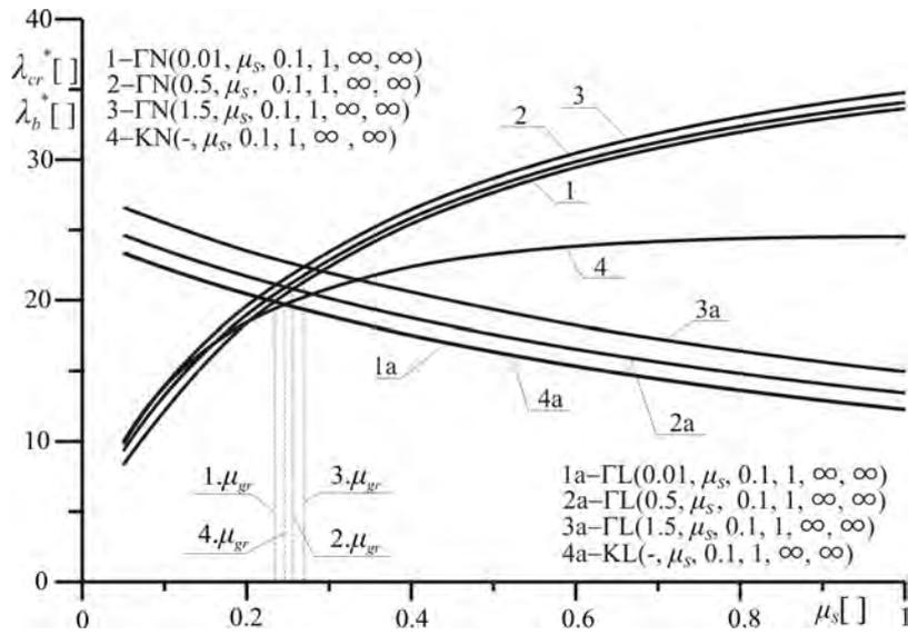
Fig. 3. The critical load parameter  $\lambda_{cr}^*$  ( $\Gamma L$  frame) and the bifurcation load parameter ( $\Gamma N$  frame)  $\lambda_b^*$  as a function of coefficient of the flexural stiffness asymmetry of frame column  $\mu_s$  for different values of coefficient of the flexural stiffness asymmetry of total system  $\mu_c$
