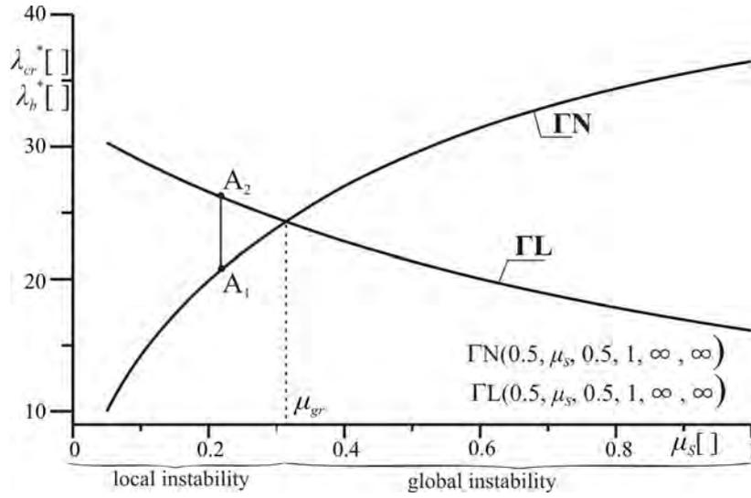
Fig. 2. The values of the critical load parameter  $\lambda_{cr}^*$  ( $\Gamma L$  frame) and the bifurcation load parameter  $\lambda_b^*$  ( $\Gamma N$  frame) in the function of coefficient of the flexural stiffness asymmetry of frame column  $\mu_s$
