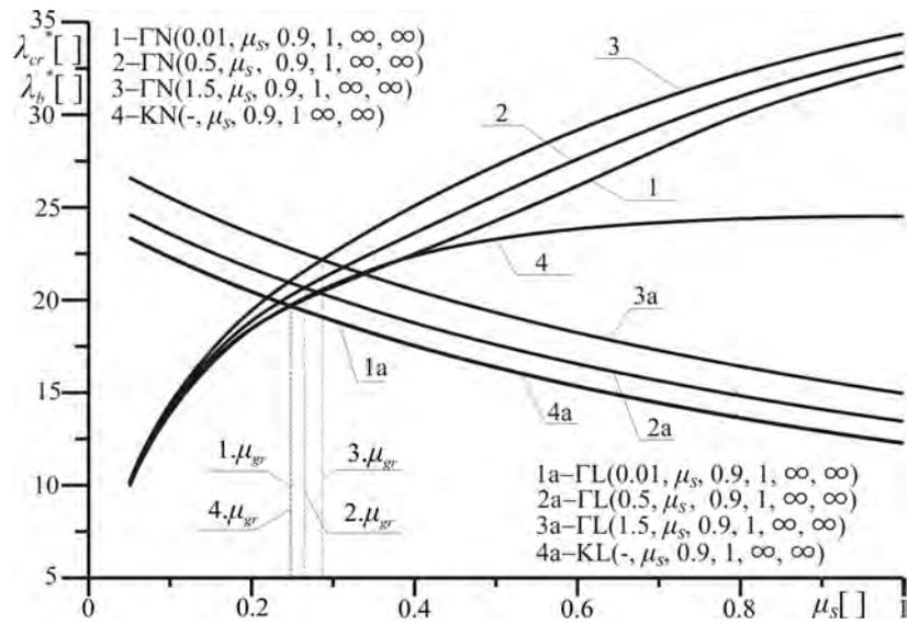
Fig. 5. The values of the critical load parameter  $\lambda_{cr}^*$  ( $\Gamma L$  frame) and the bifurcation load parameter  $\lambda_b^*$  ( $\Gamma N$  frame) as a function of coefficient of the flexural stiffness asymmetry of frame column  $\mu_s$  for selected values of coefficient of total flexural stiffness asymmetry  $\mu_C$
