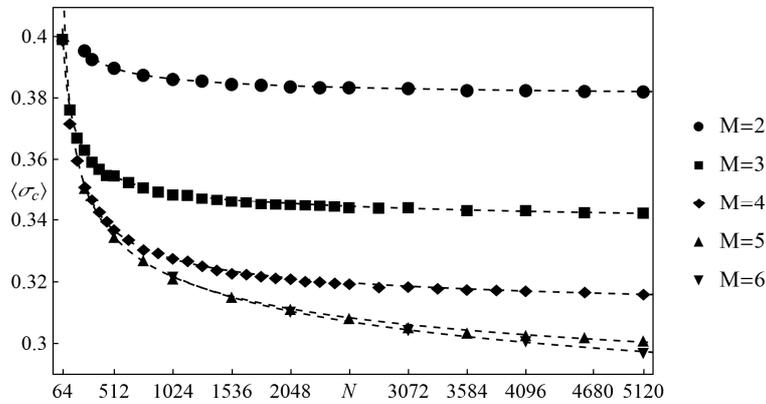
Fig. 2. The mean critical load  $\langle\sigma_c\rangle$  versus system size  $N$  for different number of hierarchy levels and  $z=4$ . The averages are taken from at least 1000 samples for each presented value. The dashed lines represent function (2) with parameters computed from simulations
