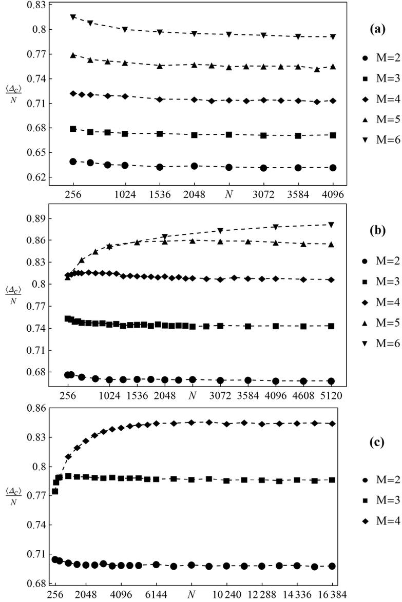
Fig. 5. The fraction of pillars destroyed during critical avalanche versus system size  $N$  for  $z = 2$  (a),  $z = 4$  (b) and  $z = 8$  (c). The data are averaged over at least 1000 realizations for each presented value
