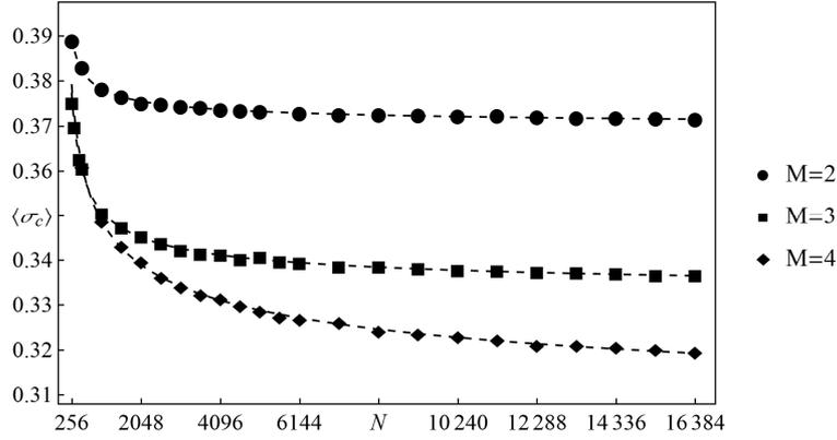
Fig. 3. The mean critical load  $\langle \sigma_c \rangle$  versus system size  $N$  for different number of hierarchy levels and  $z = 8$ . The averages are taken from at least 1000 samples for each presented value. The dashed lines represent function (2) with parameters computed from simulations
