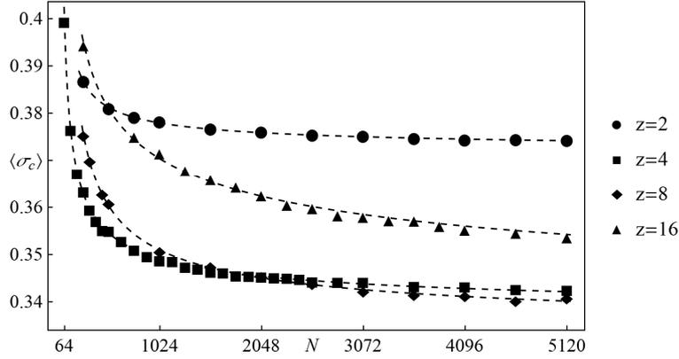
Fig. 4. The mean critical load  $\langle \sigma_c \rangle$  versus system size  $N$  for different coordination numbers and  $M = 3$ . The averages are taken from at least 1000 samples for each presented value. The dashed lines represent function (2) with parameters computed from simulations
