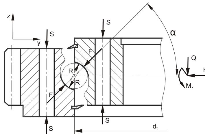
Fig. 1. One-row ball slewing bearing
