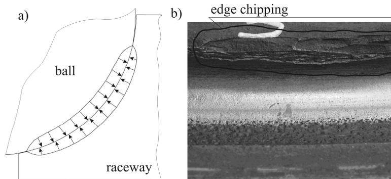
Fig. 2. The loading region of the contact zone (a), the damage of the bearing raceway (b)
