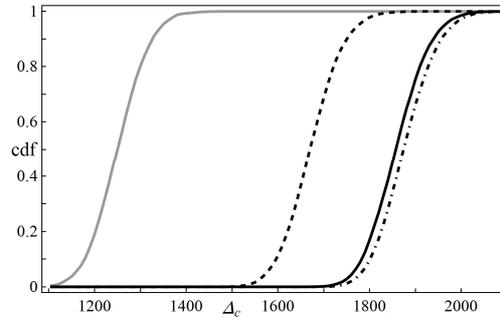
Fig. 8. The empirical cumulative distribution functions of the critical avalanche size  $\Delta_c$  in an array of  $48 \times 48$  nanopillars and  $\alpha = 2$ . Four different values of  $\gamma$  are compared:  $\gamma = 2$  (grey solid line),  $\gamma = 4$  (dashed line),  $\gamma = 8$  (black solid line),  $\gamma = 10$  (dot-dashed line). Each cdf was built on 10 000 independent configurations
