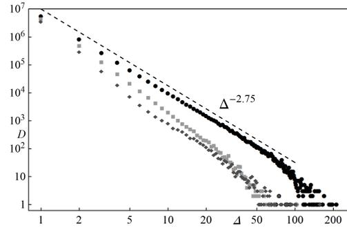
Fig. 1. The avalanche size distributions for the systems with anisotropy coefficient  $\alpha = 2$  and different values of  $\gamma$  parameter:  $\gamma = 2$  (circles),  $\gamma = 4$  (squares),  $\gamma = 8$  (diamonds). The results are obtained from 10 000 independent samples for each  $\gamma$  parameter. Size of the system  $N = 48 \times 48$  pillars
