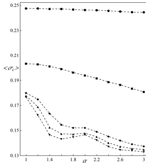
Fig. 2. The mean critical load  $\sigma_c$  versus the anisotropy coefficient  $\alpha$  for different values of  $\gamma$ :  $\gamma = 2$  (circles),  $\gamma = 4$  (squares),  $\gamma = 8$  (diamonds),  $\gamma = 10$  (up triangles),  $\gamma = 12$  (down triangles). The results are obtained from at least 2000 samples for each presented value. Size of the system  $N = 48 \times 48$  pillars
