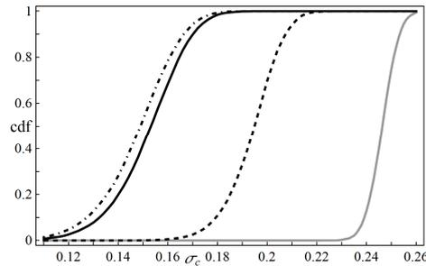
Fig. 6. The empirical cumulative distribution functions of the critical load  $\sigma_c$  in an array of  $48 \times 48$  nanopillars and  $\alpha = 2$ . Four different values of  $\gamma$  are compared:  $\gamma = 2$  (grey solid line),  $\gamma = 4$  (dashed line),  $\gamma = 8$  (black solid line),  $\gamma = 10$  (dot-dashed line). Each cdf was built on 10 000 independent configurations
