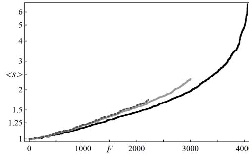
Fig. 9. The mean cluster size  $s$  versus total load  $F$  for single samples of sizes  $128 \times 128$  nanopillars and  $\alpha = 2$ . Three different values of  $\gamma$  are compared:  $\gamma = 2$  (black solid line),  $\gamma = 4$  (light grey solid line),  $\gamma = 8$  (dark grey dashed line)
