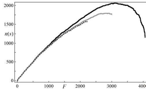
Fig. 10. The number of clusters  $n(s)$  versus total load  $F$  for single samples of sizes  $128 \times 128$  nanopillars and  $\alpha = 2$ . Three different values of  $\gamma$  are compared:  $\gamma = 2$  (black solid line),  $\gamma = 4$  (light grey solid line),  $\gamma = 8$  (dark grey dashed line)
