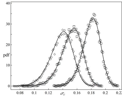
Fig. 5. The empirical probability density functions of the critical load  $\sigma_c$  in an array of  $48 \times 48$  nanopillars and  $\gamma = 8$ . Three different values of  $\alpha$  are compared:  $\alpha = 1$  (circles),  $\alpha = 2$  (squares) and  $\alpha = 3$  (diamonds). Solid lines represent skew-normally distributed  $\sigma_c$  with the location, scale and shape parameters computed from the samples. Each pdf was built on 10 000 independent configurations
