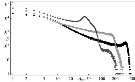
Fig. 4. The inclusive avalanche size distributions for the systems with anisotropy coefficient  $\alpha = 2$  and different values of  $\gamma$  parameter:  $\gamma = 2$  (circles),  $\gamma = 4$  (squares),  $\gamma = 8$  (diamonds). The results are obtained from 10 000 independent samples for each  $\gamma$ . Size of the system  $N = 48 \times 48$  pillars
