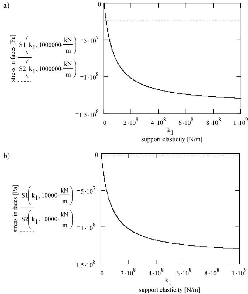
Fig. 4. The stress level in the upper face (S1 - solid line) and in the lower face (S2 - dashed line) as the function of the elasticity coefficient of the upper horizontal support  $k_1$ : a) elasticity coefficient of the lower horizontal support  $k_2 = 1\,000\,000$  kN/m, b)  $k_2 = 10\,000$  kN/m
