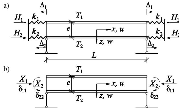
Fig. 3. The one-span basic system with the restriction of the horizontal displacement:
