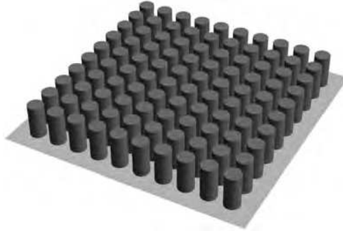
Fig. 1. An example of the set of nanopillars N = 10 \times 10 on the square lattice
