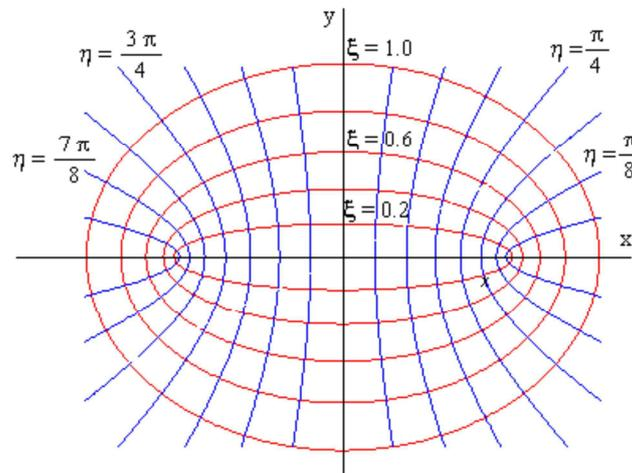
Fig. 1. Ellipses and hyperbolas in elliptical coordinates
