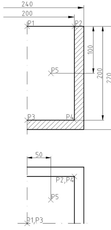
Fig. 1. Shape and dimensions of mould
