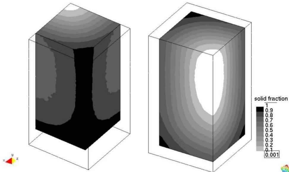
Fig. 6. Solid phase fraction distribution 125 s after pouring
