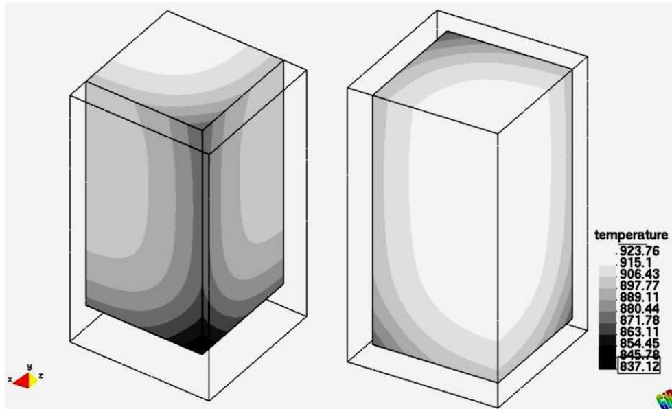
Fig. 5. Temperature field in casting 125 s after pouring
