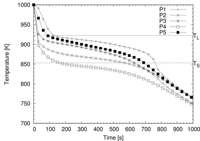
Fig. 3. Cooling curves obtained from selected points
