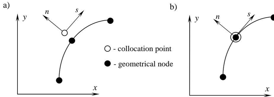
Fig. 2. Curved boundary element of constant type in non-singular and singular definition
