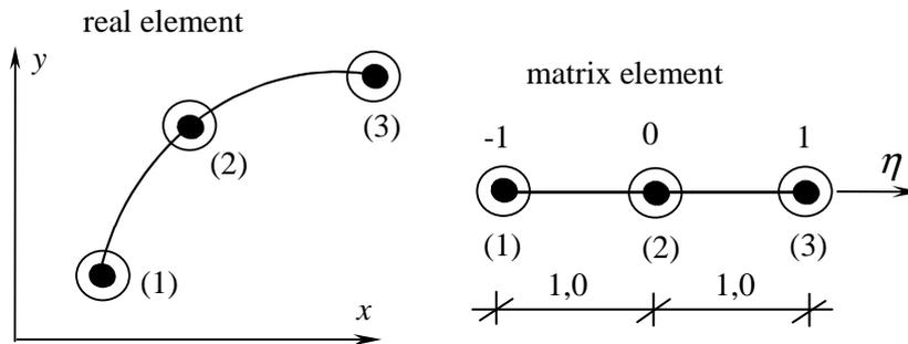
Fig. 3. Continuous, curved boundary element in singular formulation
