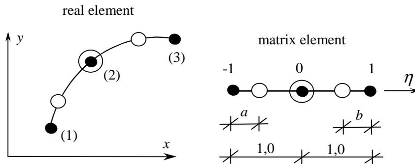
Fig. 4. Discontinuous, curved boundary element in singular formulation
