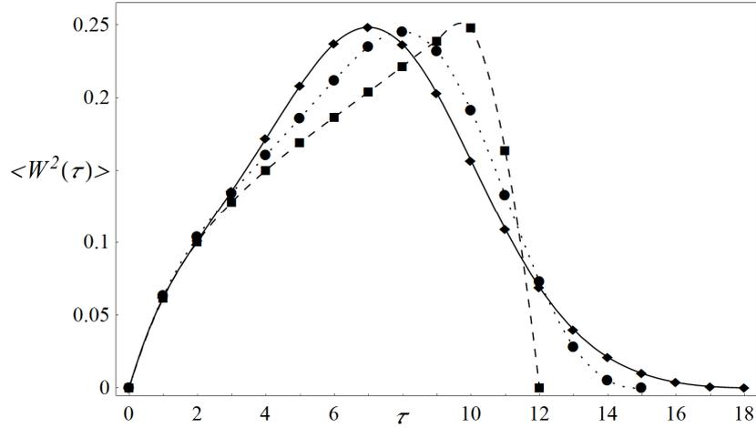
Fig. 5. The mode of surface width ( $2$ ) vs.  $\tau$ , for an array of  $2.5 \times 10^3$  pillars on the hexagonal lattice. Comparison of load transfer rules: the GLS (square), the LLS (diamond) and the VLS (circle), the modes are taken from  $10^3$  samples for each rule
