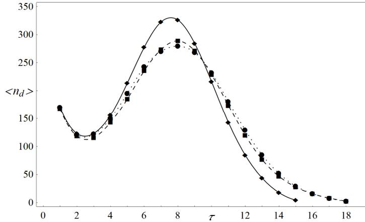
Fig. 8. Evolution of the average number of damaged elements  $\langle n_d \rangle$  with the LLS rule. Comparison of lattices: hexagonal (circle), square (square), triangular (diamond). Here,  $N \approx 2.5 \times 10^3$  and the averages are taken over  $10^3$  samples
