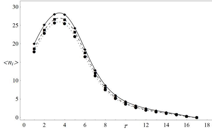
Fig. 11. Average number of intact elements  $\langle n_i \rangle$  per Voronoi region vs  $\tau$  with the VLS rule. Comparison of lattices: hexagonal (circle), square (square), triangular (diamond),  $N \approx 10^4$  and the averages are taken over  $10^3$  samples
