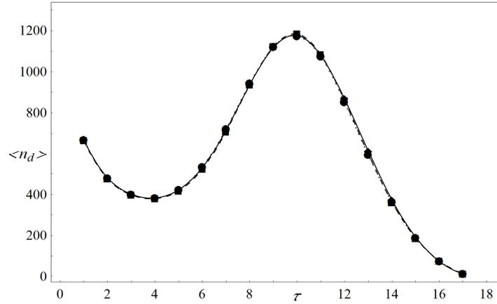
Fig. 7. Evolution of the average number of damaged elements  $\langle n_d \rangle$  with the VLS rule. Comparison of lattices: hexagonal (circle), square (square), triangular (diamond). Here,  $N \approx 10^4$  and the averages are taken over  $10^3$  samples
