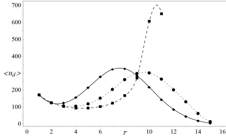
Fig. 10. Average number of damaged pillars  $\langle n_d \rangle$  vs  $\tau$  for triangular lattice. Comparison of load transfer rules: GLS (square), LLS (diamond) and VLS (circle),  $N \approx 2.5 \times 10^3$  and the averages are taken over  $10^3$  samples
