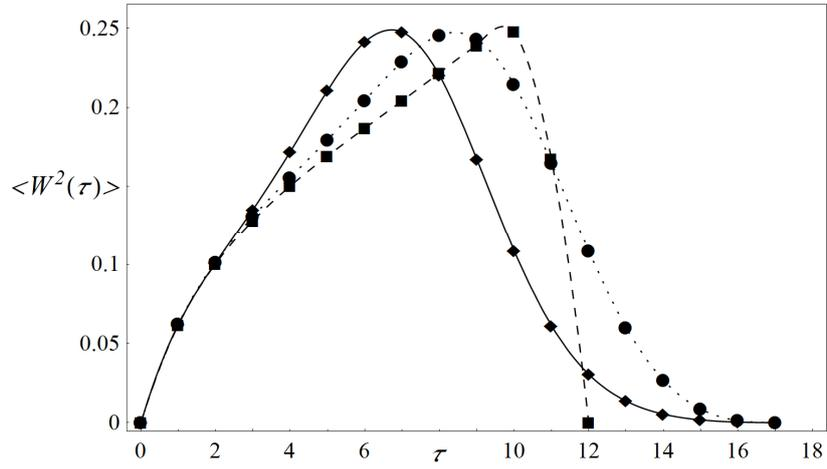
Fig. 6. The mode of surface width ( $2$ ) vs.  $\tau$ , for an array of  $10^4$  pillars on the triangular lattice. Comparison of load transfer rules: the GLS (square), the LLS (diamond) and the VLS (circle), the modes are taken from  $10^3$  samples for each rule
