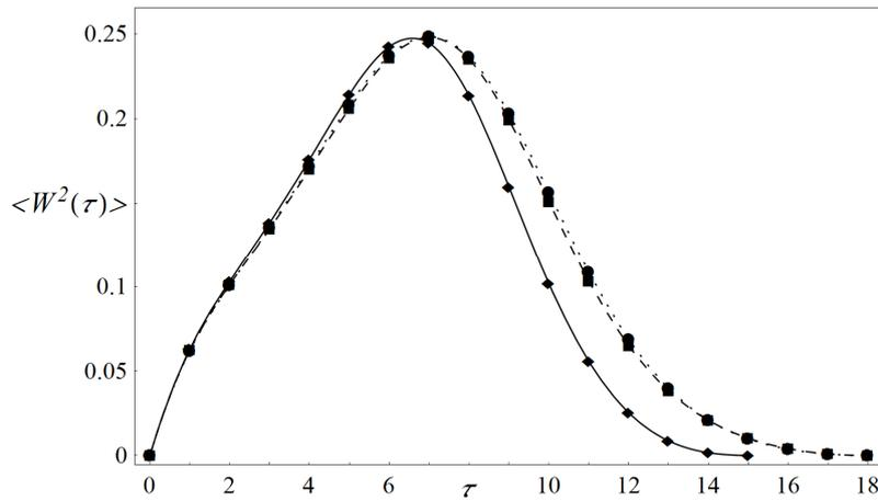
Fig. 4. The mode of surface width (2) vs.  $\tau$  with the LLS rule for an array of  $2.5 \times 10^3$  pillars. Comparison of lattice geometries: hexagonal (circle), square (square), triangular (diamond)
