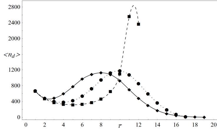
Fig. 9. Average number of damaged pillars  $\langle n_d \rangle$  vs  $\tau$  for hexagonal lattice. Comparison of load transfer rules: the GLS (square), the LLS (diamond) and the the VLS (circle),  $N \approx 10^4$  and the averages are taken over  $10^3$  samples
