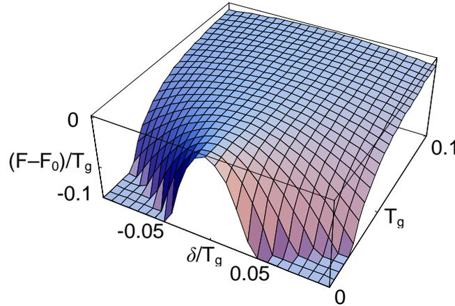
Fig. 2. Illustration relation between free energy and quantity which is characterized fluctuations of curvature and porosity of grain surface  $\delta$  and delivered energy to the system in vibration process ( $T_g$ )
