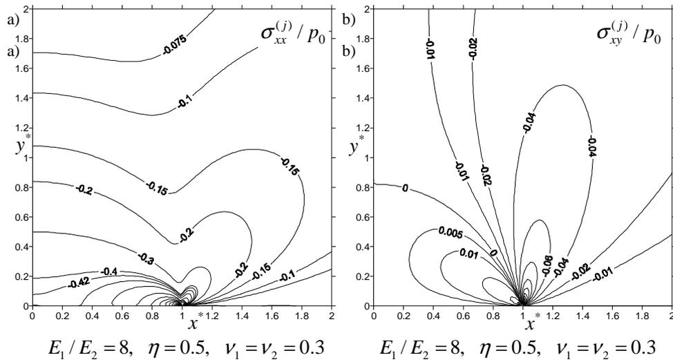
Fig. 4. The dimensionless stress distribution of lines of constant values for  $\sigma_{xx}^{(j)}$  and  $\sigma_{xy}^{(j)}$  for rectangular punch
