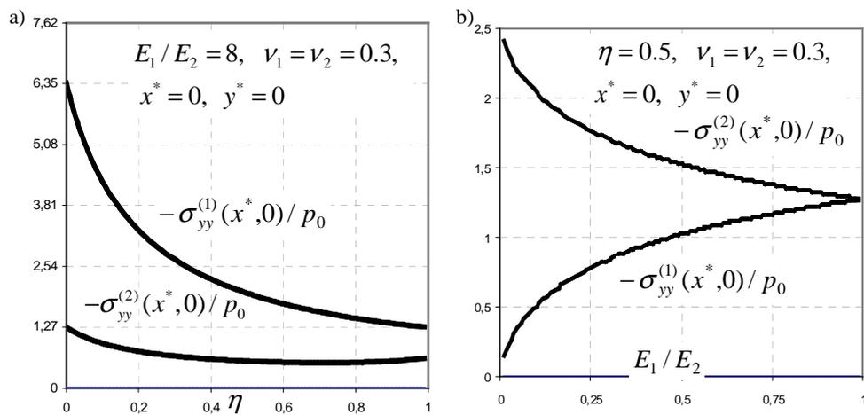
Fig. 5. The dimensionless contact pressure distribution  $-\sigma_{yy}^{(j)}(x^*, 0) / p_0$  for parabolic punch at the contact centre as a function of  $\eta$  (a) or  $E_1 / E_2$  (b)
