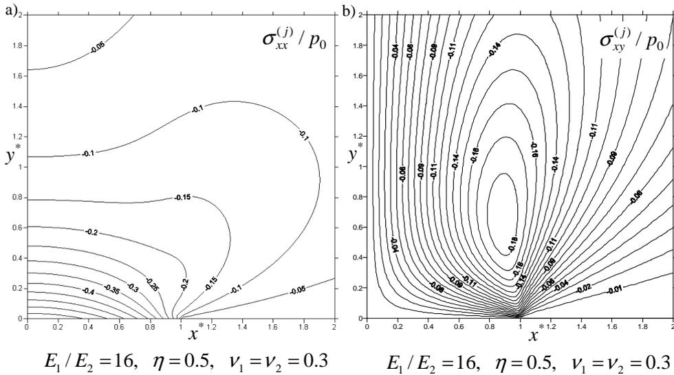
Fig. 3. The dimensionless stress distribution of lines of constant values for  $\sigma_{xx}^{(j)} / p_0$  and  $\sigma_{xy}^{(j)} / p_0$  for parabolic punch
