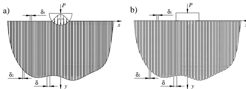
Fig. 1. A cross-section of two-layered periodically composites for two cases pressured punch:
