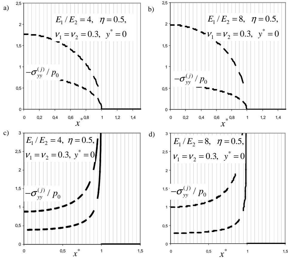
Fig. 2. The dimensionless contact pressure  $-\sigma_{yy}^{(j)}(x^*, 0)/p_0$ : a, b) parabolic punch, c, d) rectangular punch
